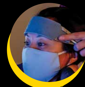
WEARABLE MONITOR NO. 1 While the study participant plays the video game, she wears a 1½-inch-wide gray band around her forehead — the fNIRS device. The headband monitors her brain activity as she moves through the game’s virtual universe, including how much oxygen she consumes.
