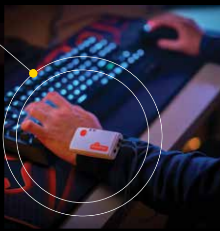
WEARABLE MONITOR NO. 2 The study participant also wears an electrodermal activity (EDA) device around the index and middle fingers of her left hand, which collects information on her skin conductance to measure emotional arousal.
