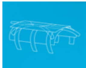
The prototype includes accordion pleats and tubes that can be used to guide surgical tools.
