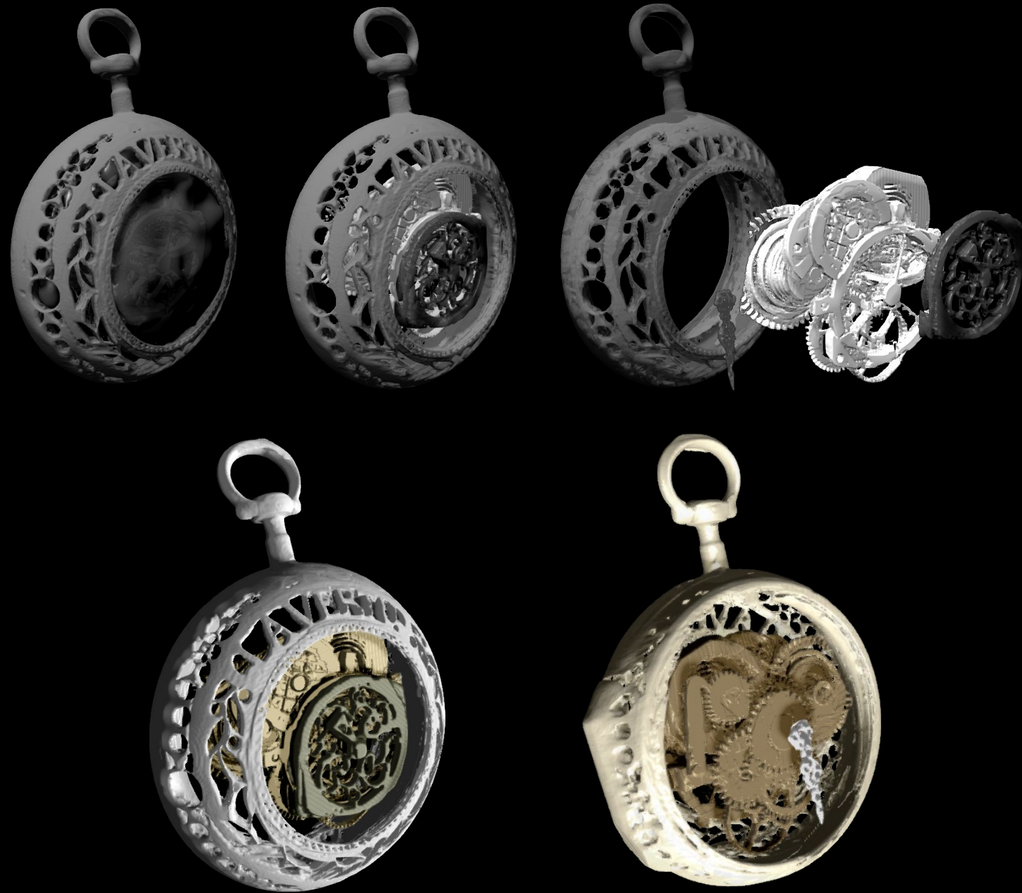
^ This set of scans of the chatelaine watch has been colorized to show the individual gears and parts using Dragonfly reconstruction software.
