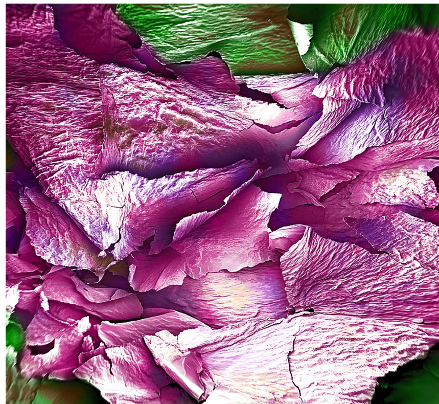
_ TINY BUT MIGHTY Scanning electron microscopy (SEM) images of the world's thinnest 1D nanofilament — just six angstroms wide. This inorganic cellulose, likened to ultra-thin spaghetti, boasts an unprecedented surface area and unique structural properties with potential applications in environmental cleanup and green hydrogen production.
