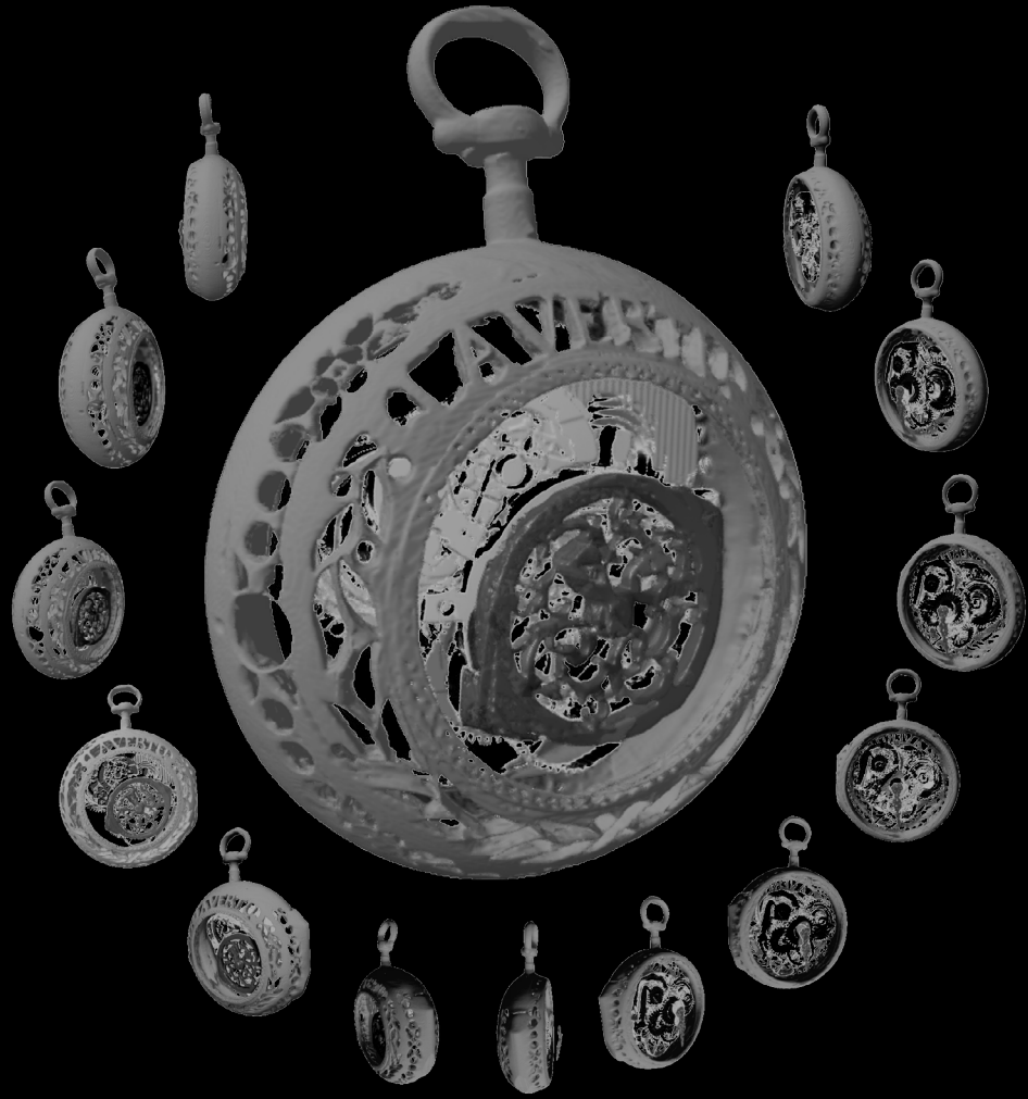
^ Drexel's nanoCT microscope produces thousands of detailed 3D scans. Researchers can rotate solid objects, zoom in on microscopic features, and isolate internal components — without harming or disassembling the object.
